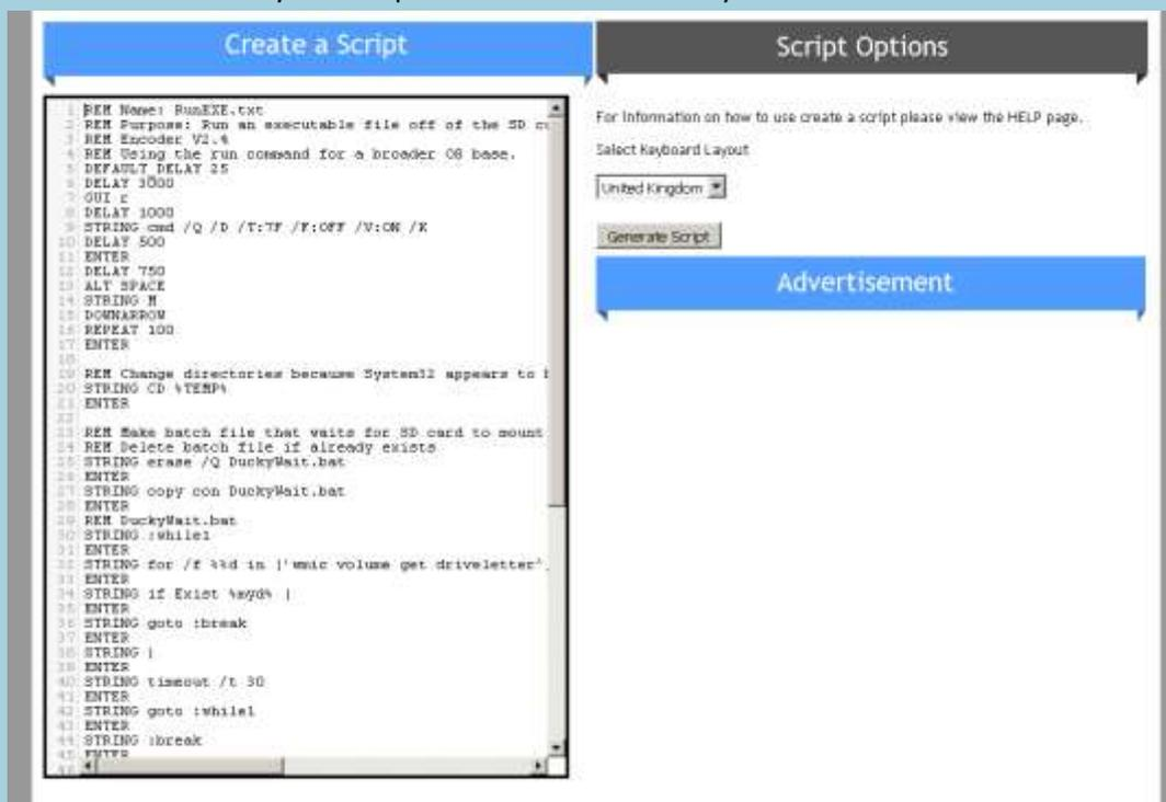
2. After you've paste your code within the encoder, select your keyboard layout, and press the generate script button. By doing this, it will allow the script to be run just like the keyboard, as this is how the hardware of the ducky ducker USB is designed.
